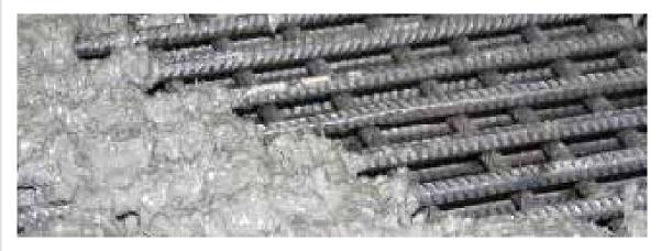
Our Ferroplan industrial floor consists of a blend of ultra high strength cement based mortars, aggregates, steel fibres and optional crack stop fibres that mix with water to give a stiff mortar. It can be laid at depths of 20-50mm with one or two layers of reinforcement mesh. Various colours and finishes are also available.
